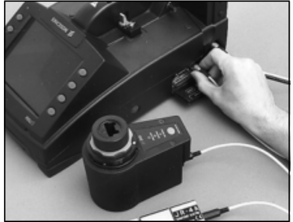
Fig. 9 - Connecting ultrasonic cleaner
