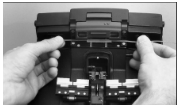
Fig. 28 - Moving ribbon from splicer to heat oven
