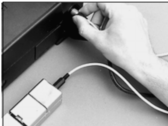
Fig. 8 - Connecting the stripper to the splicer
