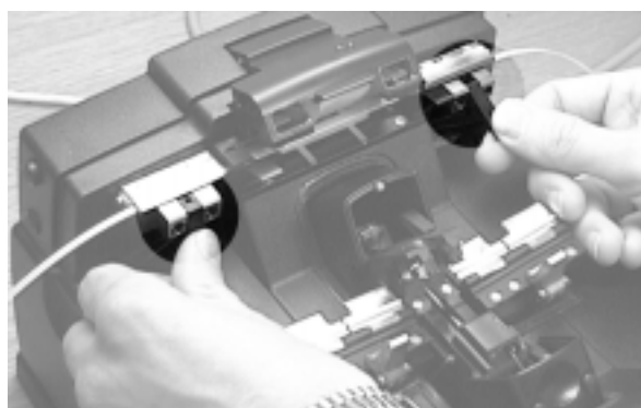
Fig. 3 - Closing the proof tester's clamps
