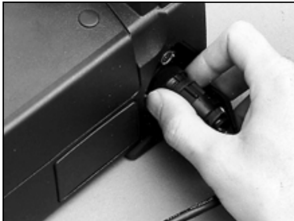
Fig. 7 - Connecting the power supply to the splicer
