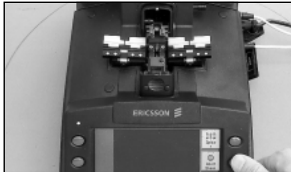
Fig. 30 - Activating the shrinking process
