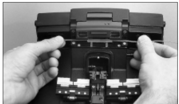
Fig. 28 - Moving ribbon from splicer to heat oven
