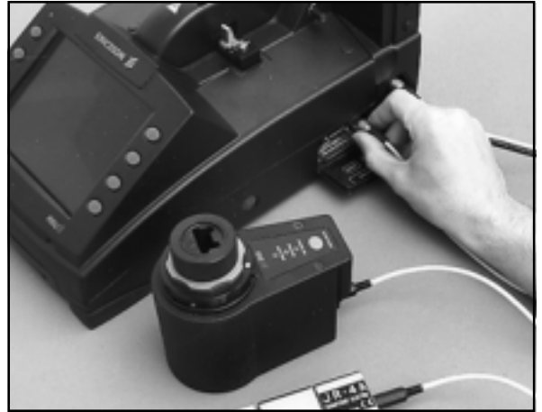
Fig. 9 - Connecting ultrasonic cleaner
